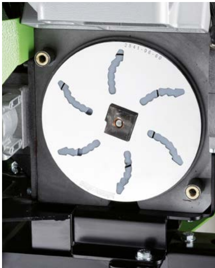
The radial slotted disk and, behind it, the spiral slotted disk
