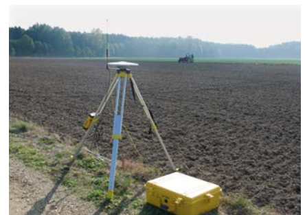
RTK station for maximum precision sowing
