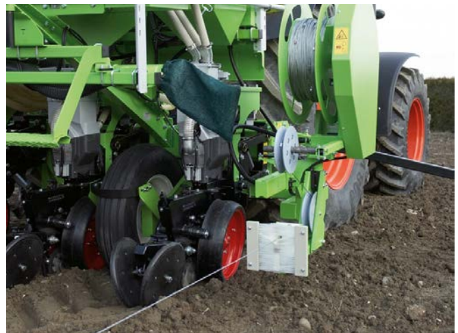
Cable trip system with cable winder
