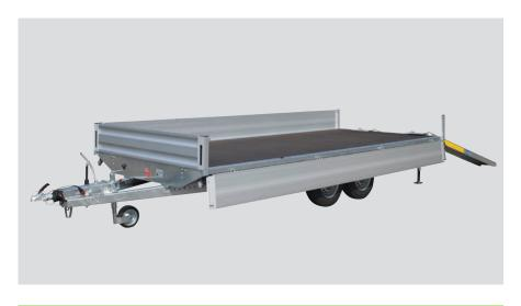
Two aluminum drive-up ramps are stored on the trailer to enable fast loading and unloading. The aluminum side walls with sunk fastenings fold down and are removable. The automatic tow coupling has both an overrun brake and an automatic reverse function.
