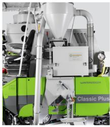
Side mounted sampler (2-man harvesting method)
